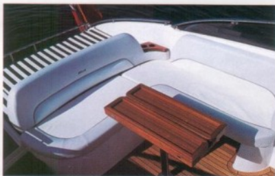
Any switch way: electrically powered sliding seat-back gives you the choice of big sunbed, or smaller sunbed and seating.
